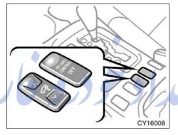
This rear height control air suspension controls the vehicle height depending on the vehicle driving conditions. Select your desired height among the "HI" (high), "N" (normal) and "LO" (low) modes with the height select switch.
