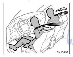
The driver and front passenger seat belt pretensioners are designed to be activated in response to a severe frontal impact. The pretensioners are also activated during vehicle rollover.
