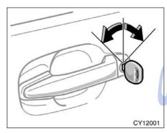
When any of the side doors and back door is unlocked with a key, the interior light, luggage compartment light, engine switch light and running board lights (on some models) will come on and remain on for about 15 seconds before fading out. (For details, see "Interior light" on page 136. "Luggage compartment light" on page 138, "Engine (ignition) switch light" on page 139 and "Running board lights" on page 140 in Section 1-5.)
