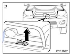
In front of the vehicle, pull up the auxiliary catch lever and lift the أرأن hood.
