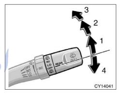
To turn on the back window wiper, twist the lever knob upward.
