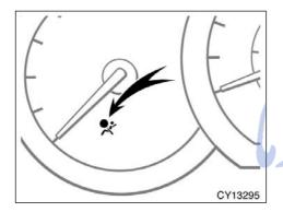
This indicator comes on when the engine switch is turned to the "ON" position. It goes off after about 6 seconds. This means the SRS side airbags and curtain shield airbags are operating properly.
