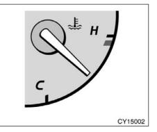
The gauge indicates the engine coolant temperature when the engine switch is on. The engine operating temperature will vary with changes in weather and engine load.
