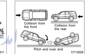
The curtain shield airbags may not activate if the vehicle is subjected to a collision from the side at certain angles, or a collision to the side of the vehicle body other than the passenger compartment as shown in the illustration.
