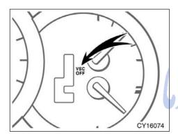
When the system is normal and the engine switch is turned to the "ON" position, the light will come on and will go off after a few seconds.
