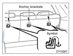
Use the anchor brackets behind the rear seatbacks to attach the top strap.
