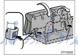
WHEN RETURNING SECOND SEATS Push the knob to unlock the seat, swing the whole seat down and swing the seatback up.
