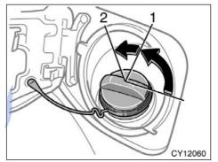
2. To remove the fuel tank cap, turn the cap counterclockwise by 90 degrees (to the pressure point 1), and When refueling, turn off the engine. then turn it an additional 30 degrees (to point 2). Pause slightly before removing it.
