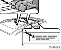
The roof luggage carrier consists of roof rails (1) attached to the roof and sliding cross rails (2).
