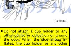
other device or object on or around the door. When the side airbag inflates, the cup holder or any other device or object will be thrown with great force or the side airbag may not activate correctly, resulting in death or serious injury. Likewise, the driver and front passenger should not hold objects in their arms or on their knees.
