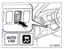
To turn on the system, briefly push the "VSC OFF" switch. At this time, the "AUTO LSD" indicator and slip indicator lights will come on.
