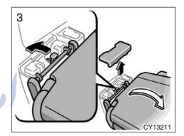
Remove the cover and push the seat lock release lever outward to unlock the seat lock, then pull up the whole seat and remove it. After removing the seat, reinstall the cover.
