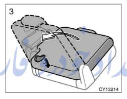
Raise the seatback while pushing down the seatback angle adjusting lever.
