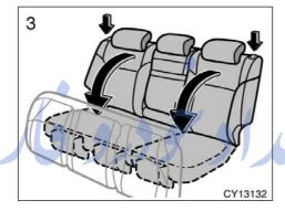
3. Push the lock release button and fold down the seatback.
