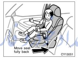
• Do not allow the child to lean his/ her head or any part of his/her body against the door or the area of the seat, front or rear pillar or roof side rail from which the side airbags or curtain shield airbags deploy even if the child is seated in the child restraint system. It is dangerous if the side airbag and/or curtain shield airbag inflate, and the impact could cause death or serious injury to the child.
