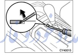
If you cannot shift the selector lever out of the "P" position to other positions even though the brake pedal is depressed, use the shift lock override button as follows:
