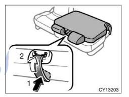
If you cannot raise the seatback because of the locked seat belt, do not try to force it. Release the lock of the seat belt in the following way.
