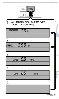
The outside temperature display (air conditioning system with "DUAL" button) and cruise information display indicates the following information.
