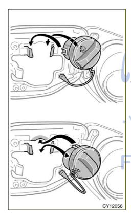
3. The removed cap can be stored on the back side of the fuel filler door.
