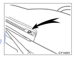
The automatic light control sensor is on the top of the driver's side instrument panel.
