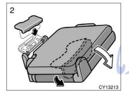
2. Pull out the seat leg from the back of the seat cushion and lock it on the anchor. Reinstall the cover.
