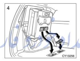
4. Remove the seat anchor covers from the back of the seat cushion, and -install them over the seat anchors.
