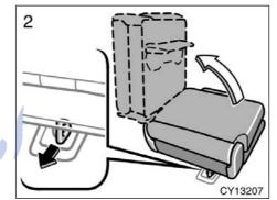
2. Unlock the seat leg by pulling the handle behind the seat, and swing
