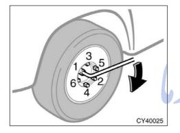
10.Lower the vehicle completely and tighten the wheel nuts.
