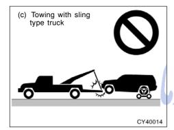
(c) Towing with sling type truck
