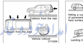
The SRS front airbags are not generally designed to inflate if the vehicle is involved in a side or rear collision, if it rolls over, or if it is involved in a lowspeed frontal collision. But, whenever a collision of any type causes sufficient forward deceleration of the vehicle, deployment of the SRS front airbags may occur.
