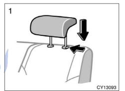
1. Lower the head restraint to the lowest position.
