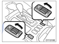
To turn on the seat heater, move the dial forward ("L" dial for the left front seat and "R" dial for the right front seat). At this time, the indicator light will illuminate to indicate the seat heater is operating.
