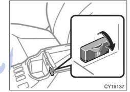
This power outlet is designed for use as a power supply for the audio device connected to the A/V input adapter.
