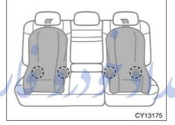
Lower anchorages for the child restraint systems complying with the FMVSS225 or CMVSS210.2 specifications are installed in the rear seats.
