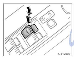
OPERATING THE DRIVER'S WINDOW Use the switch on the driver's door. Normal operation: The window moves as long as you hold the switch.
