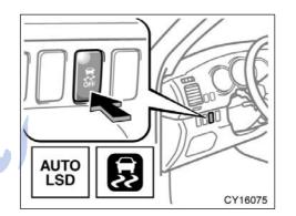
When getting the vehicle out of mud or newly fallen snow, etc., turn off the vehicle stability control system. This system that controls engine performance interferes with the process of freeing rear wheels (two-wheel drive models) or 4 wheels (four-wheel drive models).
