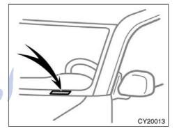
The vehicle identification number (VIN) is the legal identifier for your vehicle. This number is on the left top of the instrument panel, and can be seen through the windshield from outside.
