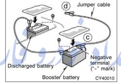
c. Connect the clamp of the negative (black) jumper cable to the negative (-) terminal on the booster battery.
