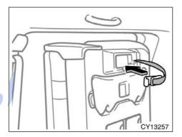
When returning the third seat to its original position, stow the holding strap in the holder in the direction shown above. Then do the above procedures in the reverse order.
