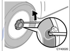
3. Remove the wheel ornament. Pry off the wheel ornament, using the beveled end of the wheel nut wrench as shown.
