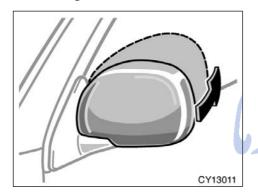
The rear view mirrors can be folded backward for parking in compact areas. To fold the rear view mirror, push backward.
