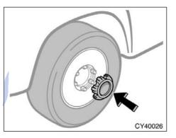
11. Reinstall the wheel ornament. Put the wheel ornament into position and then tap it firmly with the side or heel of your hand to snap it into place.
