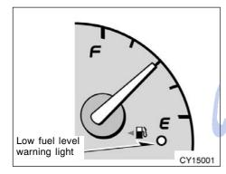
The gauge indicates the approximate quantity of fuel remaining in the tank when the engine switch is on.
