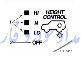
(e) Height control indicator lights1. Height control indicator lights2. Height control "OFF" indicator light
