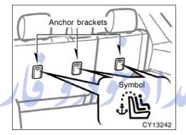
Use the anchor brackets behind the second seatbacks to attach the top strap.
