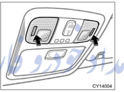
To turn on the personal lights, push the lens. To turn the lights off, push the lens once again.
