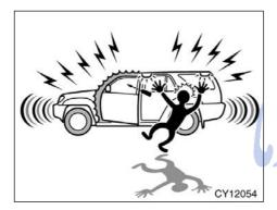
The system sounds alarm and flashes lights when forcible entry is detected. The alarm is triggered if any of the doors or hood is forcibly unlocked or opened or the battery terminal is disconnected and then reconnected when the vehicle is locked.
