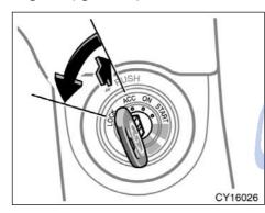
"START"—Starter motor on. The engine switch will return to the "ON" position when released.
