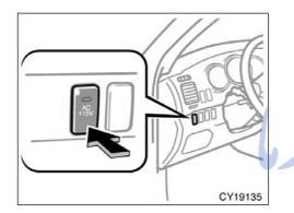
To use the power outlet, push the main switch on the instrument panel.
