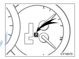
When the hill-start assist control system is operating, the slip indicator light flashes and an alarm sounds intermittently. At the same time, the stop lights and high mounted stoplight are lit.
