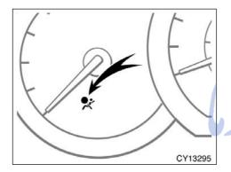
This indicator comes on when the engine switch is turned to the "ON" position. It goes off after about 6 seconds. This means the SRS front airbags are operating properly.
