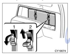
The right side of luggage compartment auxiliary box is equipped with a belt to hold the objects.
