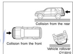
The SRS side airbags are not generally designed to inflate if the vehicle is involved in a front or rear collision, if it rolls over, or if it is involved in a lowspeed side collision.
