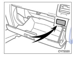
The air conditioning filter information label is placed on the upper right side of the glove box as shown and indicates that a filter has been installed.
