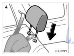
4. Replace the head restraint. Close the anchor bracket cover when the anchor bracket is not used.
