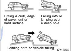
The SRS front airbags may also deploy if a serious impact occurs to the underside of your vehicle. Some examples are shown in the illustration.
