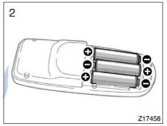
2. Remove the discharged batteries and put in the new batteries as shown.
