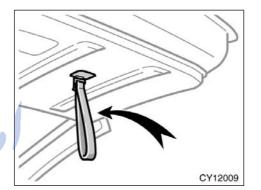
When closing the back door, the inside strap can be used to make the reach easier.
