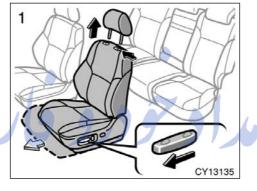
1. Remove the head restraint. Move the seat position adjusting switch forward to slide the seat further forward than the front-most position.
