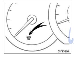
• Make sure the "RSCA OFF" indicator light is off. The curtain shield airbags will not inflate in a vehicle rollover if this indicator light is on and you may be killed or seriously injured. For details, see "Roll sensing of curtain shield airbags off switch" on page 95 in this Section.
