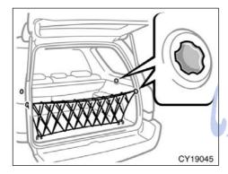
These hooks are designed to hang the cargo net.
