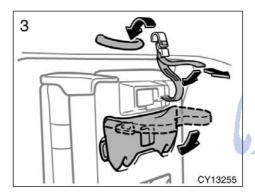
3. Stow the seat leg in the back of the seat cushion. Take the holding strap out of its holder, and attach the strap to the assist grip. Tighten the strap by pulling the end and fix it with the hook-and-loop fastener.
