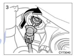
3. Install a new bulb and connector into the mounting hole and turn If the connector is tight, wiggle it. تلفن شبانه them clockwise to the front of the vehicle.
