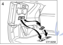
4. Remove the seat anchor covers from the back of the seat cushion, and install them over the seat anchors.
