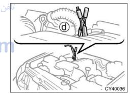
Connecting point for 4.7 L V8 (2UZ-FE) engine
