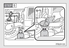
Add engine coolant if necessary.
