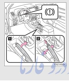
To set the parking brake, fully pull the parking brake lever while depressing the brake pedal.
