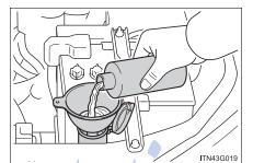
If any washer does not work, the washer tank may be empty. Add washer fluid.
