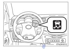
If the vehicle is in danger of slipping or if any of the drive wheels spins, the slip indicator flashes to indicate that the VSC/TRC systems are operating.
