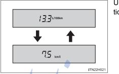
Unit for only the fuel consumption rate can be interchanged.
