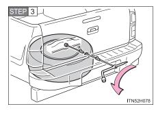
Lower the spare tire completely to the ground.
