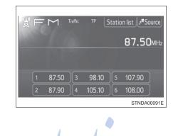
The system automatically switches to traffic information when a broadcast with a traffic information signal is received.
