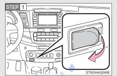
Open the cover and connect the portable audio device.
