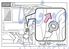
Holding a rag under the end, pull the dipstick out.
