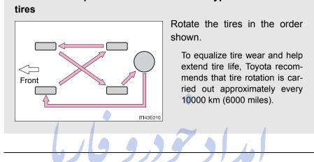
Vehicles with spare tire of the same wheel type as the installed
