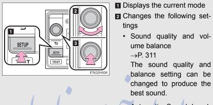
The sound quality and balance setting can be changed to produce the best sound. Automatic Sound Levelizer on/off →P. 312 **3** Selecting the mode
