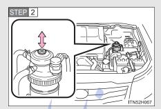
To bleed the fuel system, operate the priming pump until you feel more resistance.
