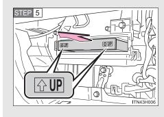
Remove the filter and replace it with a new one.
