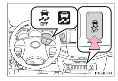
To turn the TRC and VSC systems off, press and hold the button for more than 3 seconds while the vehicle is stopped.
