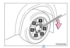
Tightening torque: 105 N•m (10.7 kgf•m, 77 ft•lbf)
