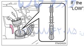
If the washer fluid level is at "LOW", add washer fluid.
