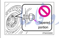
Be sure to install the wheel nuts with the tapered end facing inward. Installing the nuts with the tapered end facing outward can cause wheel to break and eventually cause a wheel to come off while driving, which could lead to an accident resulting in death or serious injury.
