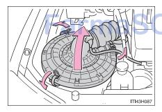
Release the clips of the air cleaner filter cover, and remove the cover to allow easy access to the light bulbs.
