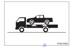
If you use chains or cables to tie down your vehicle, the angles shaded in black must be  $45^{\circ}$ .
