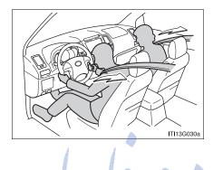
The pretensioner helps the seat belt to quickly restrain the occupant by retracting the seat belt when the vehicle is subjected to certain types of severe frontal collision or side collision (vehicles with SRS side airbags and curtain shield airbags).
