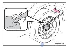
Pry off the wheel ornament, using the beveled end of the wheel nut wrench as shown.
