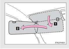
To set the visor in the forward position, flip it down.
