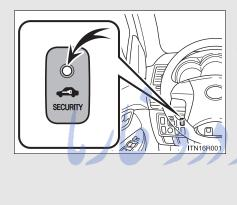
The indicator light flashes after the key has been removed from the engine switch to indicate that the system is operating.
