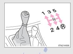
Fully depress the clutch pedal before operating the shift lever, and then release it slowly.
