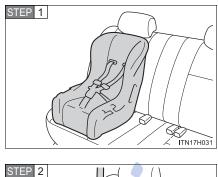
Place the child restraint system on the seat facing the front of the vehicle.
