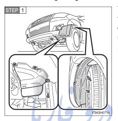
To allow enough working space, turn the steering wheel to the opposite side of the bulb to be replaced.
