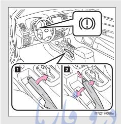
■ To set the parking brake, fully pull the parking brake lever while depressing the brake pedal.
