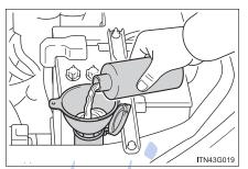
If any washer does not work, the washer tank may be empty. Add washer fluid.
