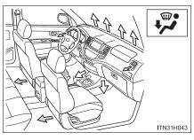
Air flows to the feet and the windshield defogger operates.
