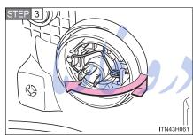
Release the bulb retaining spring.
