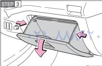
Push in each side of the glove box to disconnect the claws.
