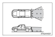
The area covered by the camera is limited. Objects which that are close to either corner of the bumper or under the bumper cannot be seen on the screen.
