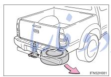
If the tire is still underneath the vehicle, leave the vehicle jacked up and use a tool to pull the tire out.
