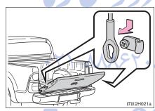
Release the brackets on the support cables from the lugs on both sides as shown in the illustration.
