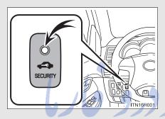
The indicator light flashes after the key has been removed from the engine switch to indicate that the system is operating.
