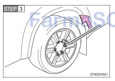
Slightly loosen the wheel nuts (one turn).
