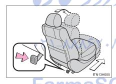
Depress the release pedal and fold down the seatback. The seat will slide forward.
