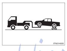
Vehicles with automatic transmission: Use a towing dolly under the rear wheels.
