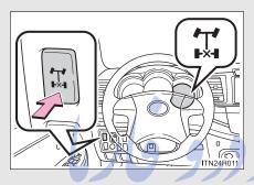
Press the rear differential lock switch to lock the rear differential.
