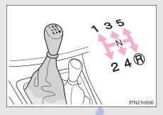
Fully depress the clutch pedal before operating the shift lever, and then release it slowly.
