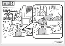
Add engine coolant if necessary.
