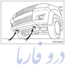
If a tow truck is not available in an emergency, your vehicle may be temporarily towed using a cable or chain secured to the emergency towing eyelet(s). This should only be attempted on hard surfaced roads for short distances at low speeds.
