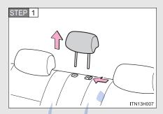
Remove the center head restraint.
