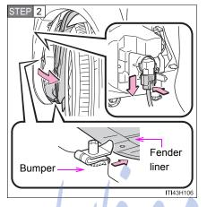
Partly remove the fender liner and unplug the connector while pressing the lock release.
