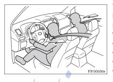
The pretensioner helps the seat belt to quickly restrain the occupant by retracting the seat belt when the vehicle is subjected to certain types of severe frontal collision or side collision (vehicles with SRS side airbags and curtain shield airbags).
