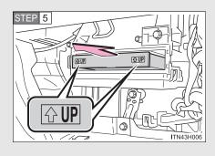
Remove the filter and replace it with a new one.
