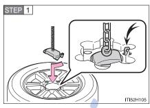
Lay down the tire with the outer side facing up, and hook the holding bracket as shown in the illustration.
