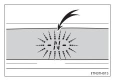
If the direction display on the compass flashes, circling calibration needs to be performed.
