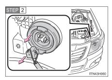
Unplug the connector and remove the rubber cover.
