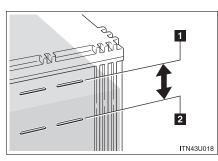
Check that the level is between the upper and lower lines.
