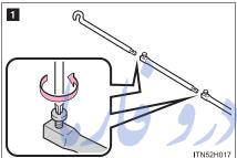
**1** Loosen the bolts using a screwdriver.
