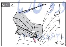
Run the seat belt through the child restraint system and insert the plate into the buckle. Make sure that the belt is not twisted. Keep the lap portion of the belt tight.
