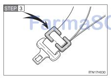
Install a locking clip near the plate of the lap and shoulder belt by inserting the lap and shoulder webbing through the recesses of the locking clip.
