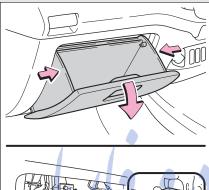
Open the glove box. Push in each side of the glove box to disconnect the claws.
