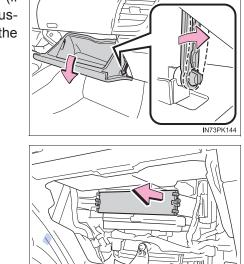
6 Remove the air conditioning filter and replace it with a new one.
