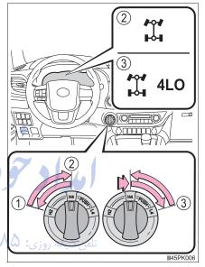
Use this for maximum power and traction. Use "L4" for climbing or descending steep hills, off-road driving, and hard pulling in sand, mud or deep snow.
