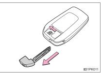
After using the mechanical key, store it in the electronic key. Carry the mechanical key together with the electronic key. If the electronic key battery is depleted or the entry function does not operate properly, you will need the mechanical key. ( $\rightarrow$ P. 519)
