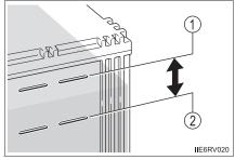
If there are not lines on the side of the battery: Check the fluid level as follows.
