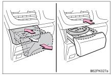
Press in and pull the cup holder, and push the cup tray.
