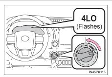
If the shift lever is shifted to other than N while the low speed four-wheel drive indicator light is flashing, gear noise may be caused. Immediately shift the shift lever to N and wait until switching the transfer mode is completed.
