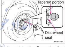
Tapered portion Tapered portion Discwheel seat
