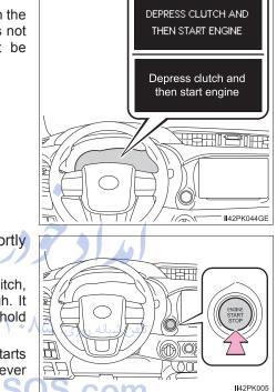
Press the engine switch shortly and firmly.
