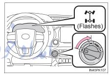
Reduce the vehicle speed to less than 100 km/h (62 mph), or return the front-wheel drive control switch to H2 and try step 1 again.
