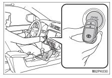
3 Firmly depress the brake pedal.
