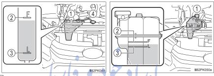
**5** Add engine coolant if necessary. ( $\rightarrow$ P. 636)
