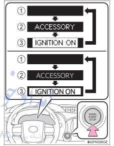
\*: If the shift lever is in a position other than P when turning off the engine, the engine switch will be turned to ACCESSORY mode, not to off (vehicles with automatic transmission only).
