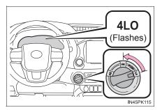
If the clutch pedal is released while the low speed four-wheel drive indicator light is flashing, gear noise may be caused. Immediately depress the clutch pedal firmly and wait until switching the transfer mode is completed.
