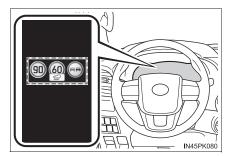
When other than the driving assist system information is selected, a speed limit sign, a highway sign or an all canceled sign can be displayed. (→P. 136)
