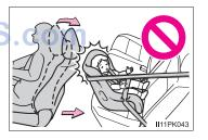
Child restraint system fixed with a seat belt (except for Kazakhstan)
