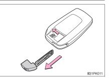
After using the mechanical key, store it in the electronic key. Carry the mechanical key together with the electronic key. If the electronic key battery is depleted or the entry function does not operate properly, you will need the mechanical key.  $(\rightarrow P. 603)$
