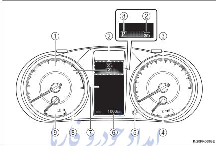
The units used on the speedometer may differ depending on the target region, and the positions of the outside temperature and shift position indicators differ depending on vehicles.
