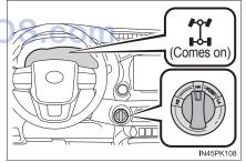
The four-wheel drive indicator light may not stop flashing if the frontwheel drive control switch is turned from H2 to H4 while the vehicle is stopped. In this case, perform any of the followings.
