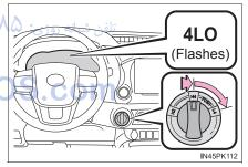
If the shift lever is shifted to other than N while the low speed four-wheel drive indicator light is flashing, gear noise may be caused. Immediately shift the shift lever to N and wait until switching the transfer mode is completed.
