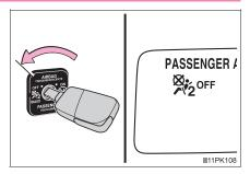
Insert the mechanical key into the cylinder and rotate to the "OFF" position.
