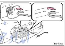
3 Lower the spare tire completely to the ground.
