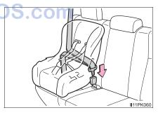
3 If your child restraint system is not equipped with a lockoff (a seat belt locking feature), secure the child restraint system using a locking clip.
