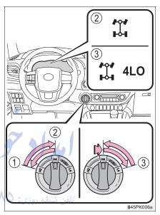
Use this for maximum power and traction. Use L4 for climbing or descending steep hills, off-road driving, and hard pulling in sand, mud or deep snow.
