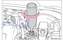
4 Push down on the bottle. Y + AdBlue™ will begin to be refilled. Refill AdBlue™ slowly so that it does not spill. Do not remove the bottle until it is empty.
