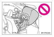
Vehicles with front passenger occupant classification system: Never use a rear-facing child restraint system on the front passenger seat when "ON" of the "PASSENGER AIR BAG" indicator is illuminated. (→P. 57) The force of the rapid inflation of the front passenger airbag can cause death or serious injury to children in the event of an accident.
