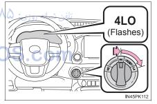
If the clutch pedal is released while the low speed four-wheel drive indicator light is flashing, gear noise may be caused. Immediately depress the clutch pedal firmly and wait until switching the transfer mode is completed. 4 Check that the low speed four-wheel drive indicator light comes on.
