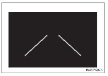
Indicates that the system is recognizing white (yellow) lines. When the vehicle departs from its lane, the white line displayed on the side the vehicle departs from flashes. Indicates that the system is not able to recognize white (yellow) lines or is temporarily canceled.
