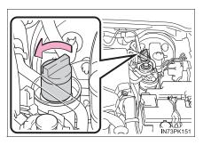
Insert a bottle of AdBlue™ and fully tighten it.
