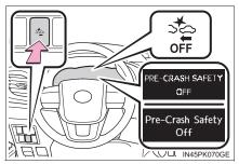
The system is enabled each time the engine switch is turned to the "ON" position (vehicles without smart entry & start system) or IGNITION ON mode (vehicles with smart entry & start system).
