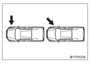
The SRS side and curtain shield airbags do not generally inflate if the vehicle is involved in a rear collision, if it rolls over, or if it is involved in a low-speed side or low-speed frontal collision.
