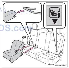
3 After installing the child restraint system, rock it back and forth to ensure that it is installed securely. (→P. 88)
