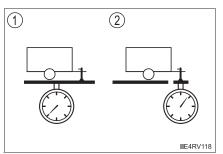
When the total trailer weight is over 2000 kg (4409 lb.), a friction stabilizer (sway control device) is required.
