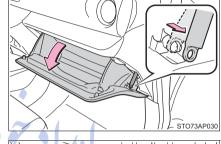
3 Push in each side of the glove box to disconnect the upper claws.
