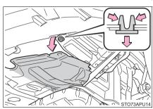
3 Partly remove the fender liner.
