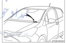
This number is also on the Certification Label on the driver's side of the center pillar.
