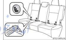
Seat belts equipped with a child المانه روزي: الك locking \ mechanism \ الله روزي: الك restraint (ALR/ELR belts except driver's seat belt) (→P. 26)
