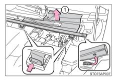
2 Remove the battery terminal cover and then the fuse box cover.
