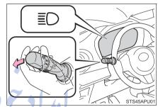
2 Press the Automatic High Beam switch.
