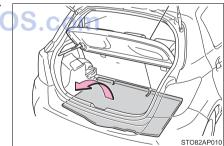
3 Loosen the center fastener that secures the spare tire.
