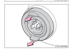
3 Release the bulb retaining spring.
