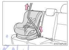
If the child restraint has a top tether strap, the top tether strap should be latched onto the top tether strap anchor. (→P. 63)
