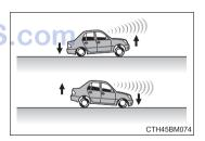
When the sensor is misaligned due to a strong impact being applied to the sensor, etc.
