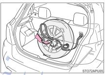
Put the center portion of the belt onto the rear center head restraint position and then return the rear center head restraint.
